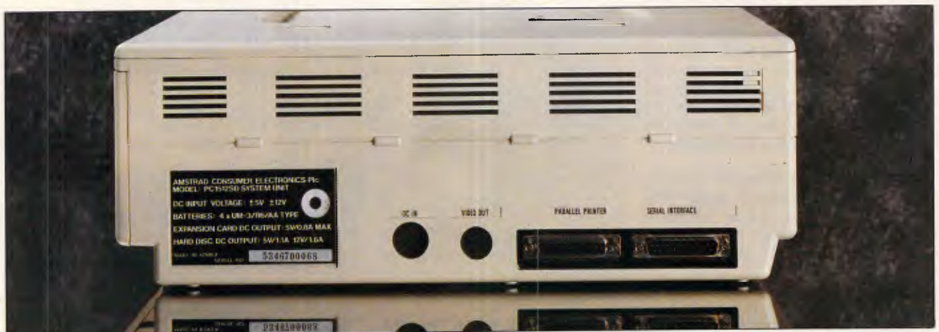
From left to right: two sockets for the monitor cables, and the parallel and serial ports respectively
